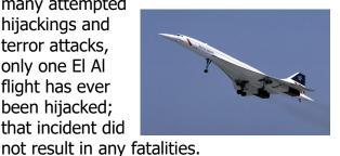
The Aérospatiale/BAC **Concorde** is a British—French turboiet-powered supersonic 2003. It had a maximum speed over twice the speed of sound, at Mach 2.04 (1,354 mph or 2,180 km/h at cruise altitude), with seating for 92 to 128 passengers. First flown in 1969, Concorde entered service in 1976 and continued flying for the next 27 years. It is one of only two supersonic transports to have been operated commercially; the other is the Soviet -built Tupolev Tu-144, which operated in
